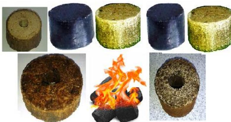
the mixed composition briquettes containing Tkibuli coal wastes, they are characterized by high thermal capacity (table 1), so they can be used in a relatively powerful industries, energetic, drying equipment, etc. Stability of this briquette depends mainly on pressure and temperature conditions of pressing.
